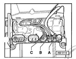
Measure resistance at connector -C- between contacts 1 and 2.
