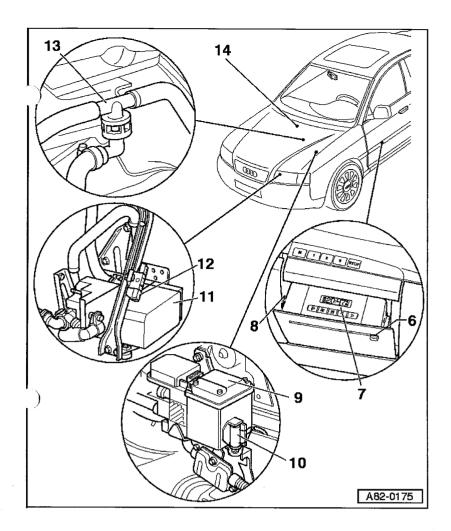
The auxiliary heater is fitted with the following electrical components:
