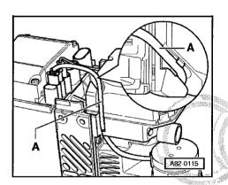
Lay wiring -A- in groove as shown.
