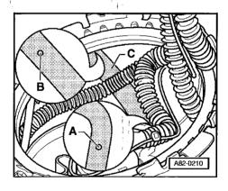
◆ Fuel pipe -C- cannot be replaced. However, to avoid having to replace the entire fuel tank in the event of a complaint on vehicles provided with hole -A-, an additional hole (max. diameter 2 mm) can be made at the highest point of fuel pipe -C- still accessible (rigid light grey pipe).
