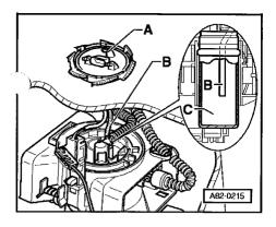
♦ If auxiliary heater functions properly when fuel tank is completely full, but problems are encountered when tank is only partially filled (fault message "No flame" or "Repeated flame interruption"), this is an indication of incorrect routing of suction pipe -B-.
