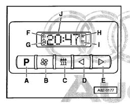
Checking and altering operating time set for auxiliary heater on pre-selection clock
