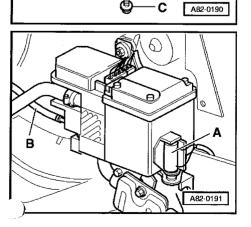
Detach series resistor -A- from auxiliary heater.
